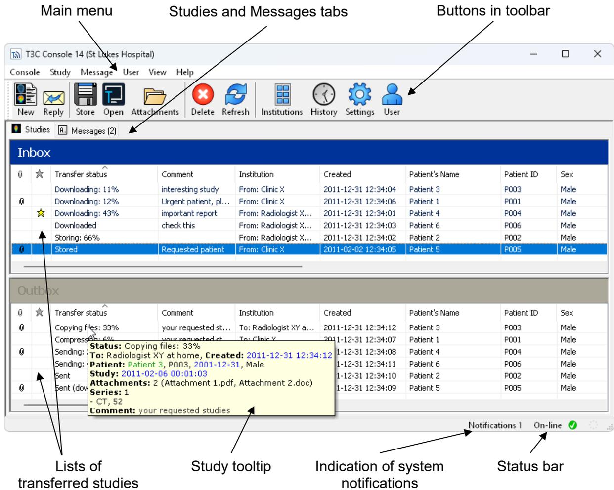
Figure 1 – T3C Console main window
